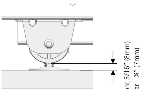
Minimum height adjustment for leveling
