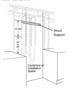
Secure the wood support to 2 or more vertical studs, using at least 2 of the 4 supplied long screws.
