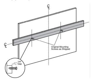
Adjust depth of original mounting srcrews in the wood support until they protrude 1/4" forward. This 1/4" gap will provide clearance to hang the hood.
