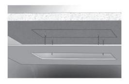
Make 4 holes in the ceiling according to the dimensions as shown in Fig. 4, place the metric plugs provided in the holes.
