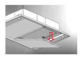
To achieve the complete opening of panels, you need to release the safety chains, by using the appropriate spring catches.
